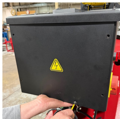
(b) Lift the access panel while installing bolts.
