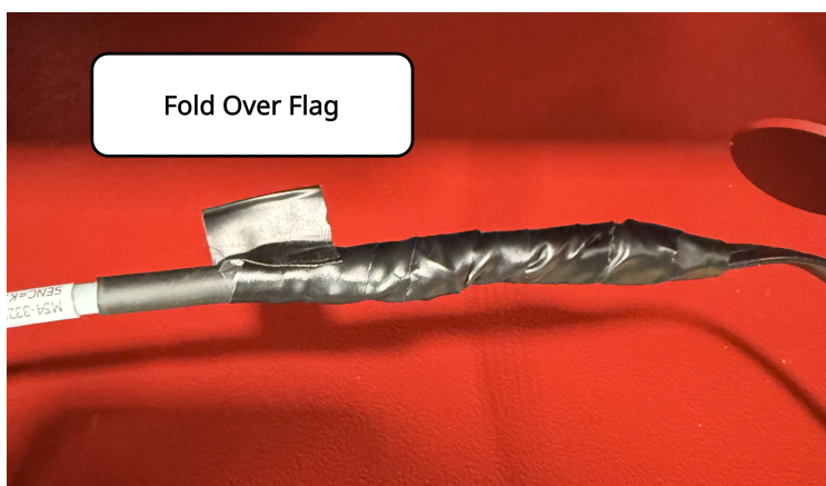
Figure 5.4: Connect the old cable to the new encoder cable with tape.
