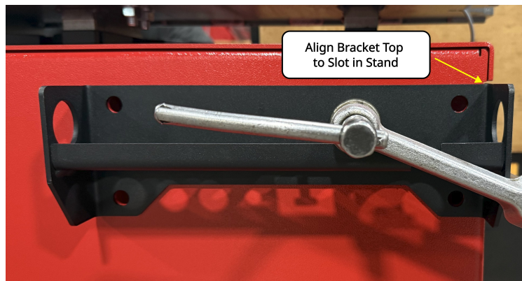
Figure 4.2: Handle bracket aligns with laser cut slot in side panel.
