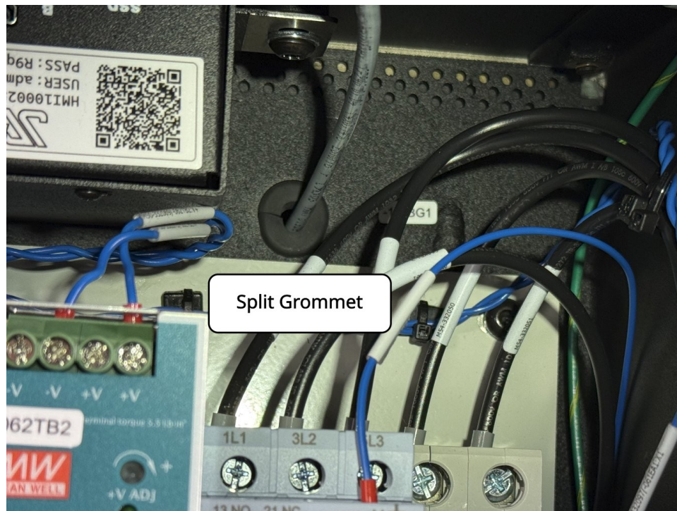
Figure 6.8: Install the encoder cable protection grommet.
