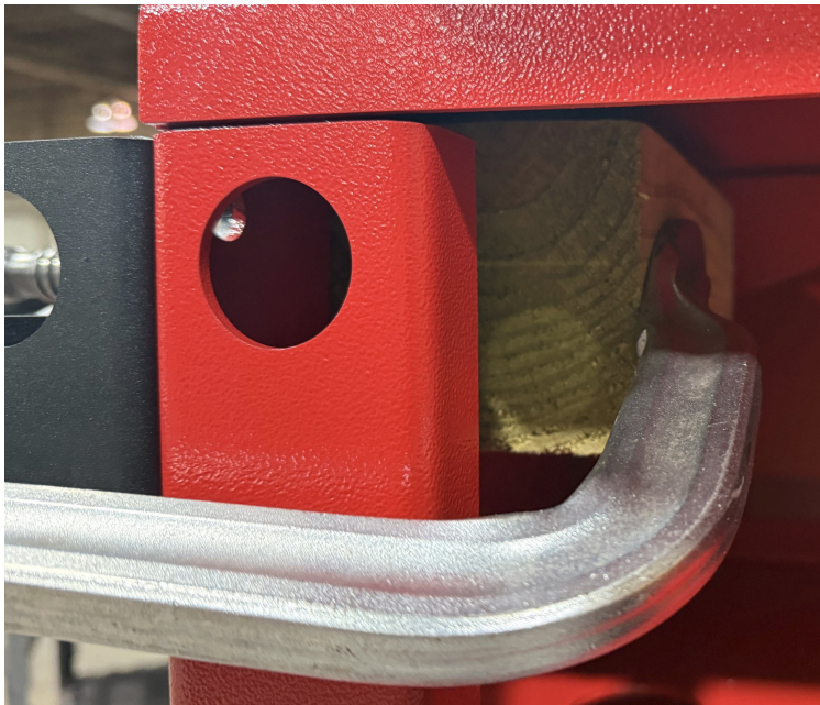
Figure 4.3: Clamp the bracket to the side with a spacer block inside the cabinet.
