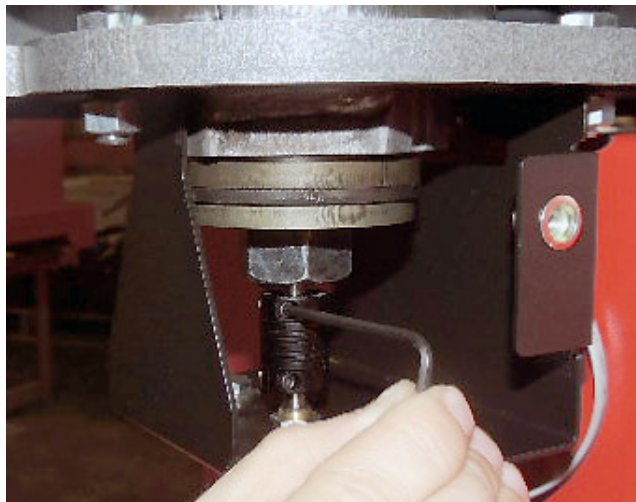
Figure 10.2: Adjusting Encoder Coupling
