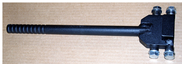
Figure 4.12: The Handle Assembly with Bolts, Washers and Sleeves
